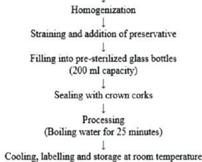
Fig. 1. Schematic figure showing flow sheet for processing of raw materials, suitable blend proportions and preparation of RTS drink variants
